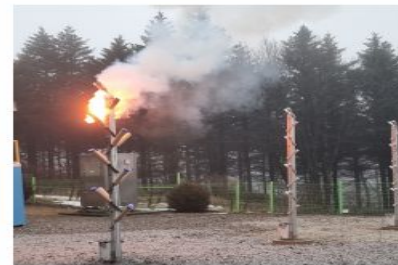
Figure 3: Total of 15 \text{CaCl}_2 Tarhunna MK1 (Cloud Technologies GmbH) seeding flares were installed and burned during the field experiment.
